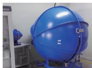
Integrating Sphere (for Testing LED Luminous)
