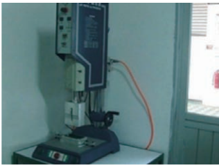
Ultrasonic Welding for Sealing Plastic Case
