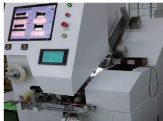
3 in 1 Auto inspection machine (Flatness/Visual/Taping)
