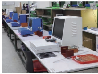
SMD Flatness Inspection
